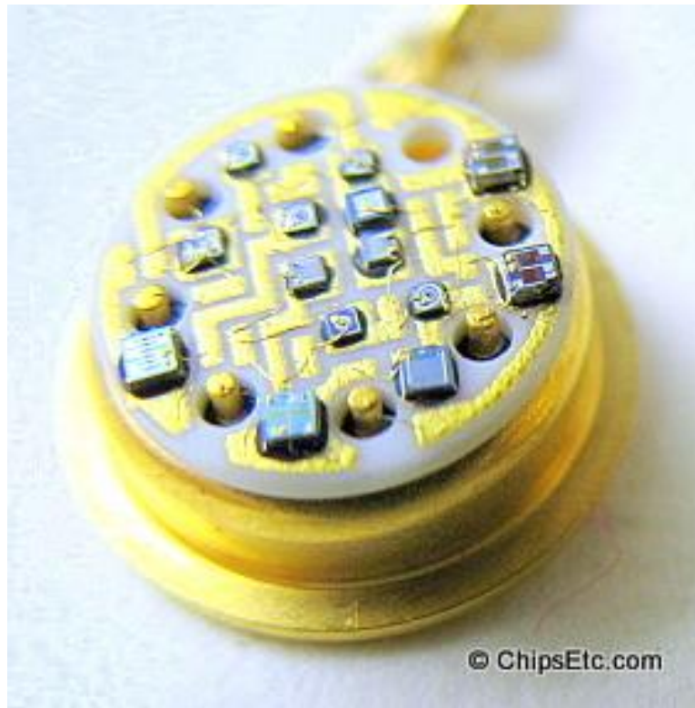
Figure 29: Inside a vintage hybrid module. [Attribution]
