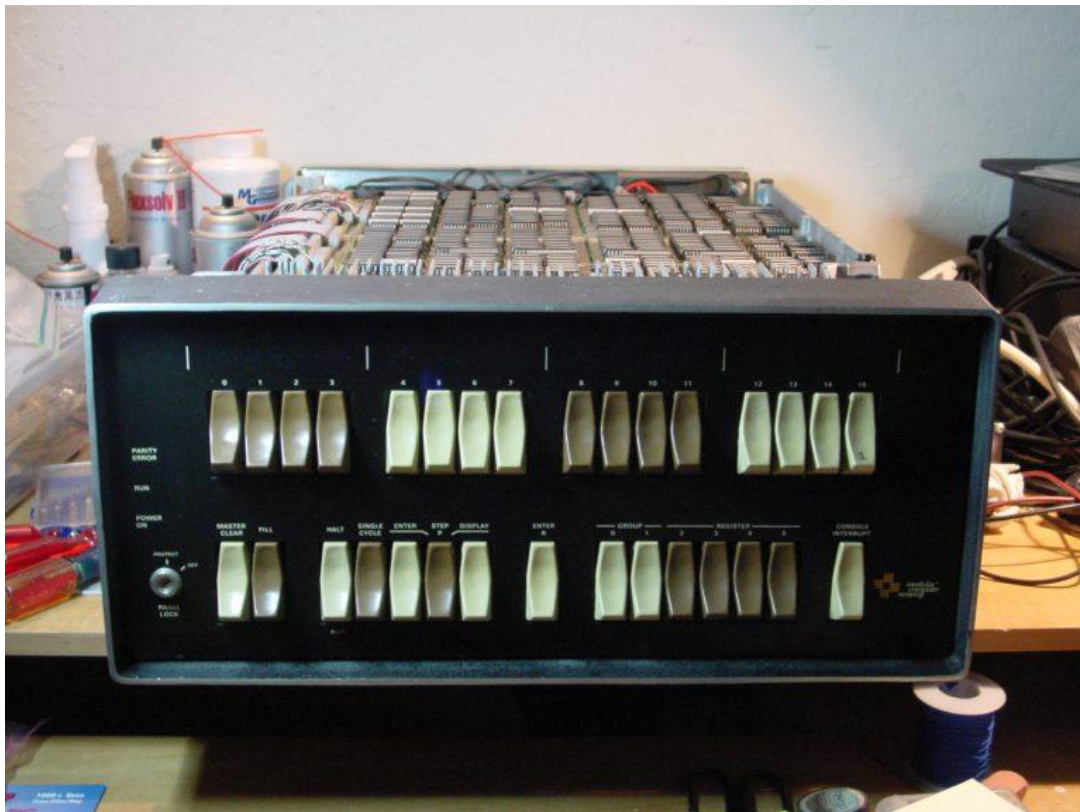
Figure 25: Modcomp II minicomputer. The keys allow a short bootstrap or test program to be entered into memory manually. [Attribution]
